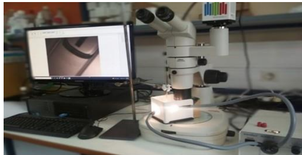
Experimental setup of pendant drop method
